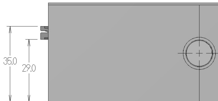
Figure 15: Argus 2000 Connector Mounting Location (front view).
